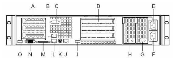
Figure 3: Chassis Back I/O Ports and Features
